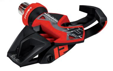
Automatic pre-opening of engagement mechanism Hollow titanium axle and carbon body with flexible carbon blade Oversized pedal platform 700 mm<sup>2</sup> with interchangeable aluminum plate Adjustment of angular sensations, or "feel" Q-Factor adjustment — setting of lateral foot position BIOPOSITION Concept — minimal distance sole to pedal axle Angular float (+/-5°) and lateral float (2.5 mm) Release angle: 15° Weight: 155 g/pair
