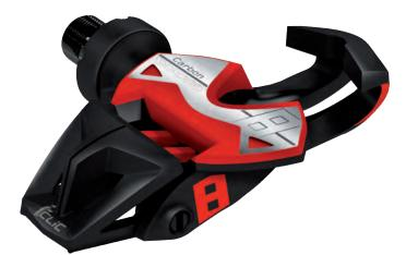
Automatic pre-opening of engagement mechanism Hollow steel axle and carbon body with flexible carbon blade Oversized pedal platform 700 mm<sup>2</sup> with interchangeable stainless steel plate Adjustment of angular sensations, or "feel" Q-Factor adjustment — setting of lateral foot position BIOPOSITION Concept — minimal distance sole to pedal axle Angular float (+/-5°) and lateral float (2.5 mm) Release angle: 15° Weight: 195 g/pair
